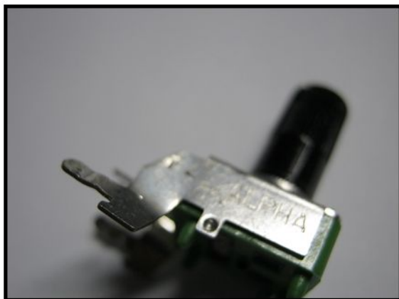
Frame 'foot' bent outward OR Frame foot cut off
